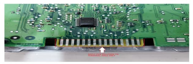
Re-pond terminals and gently take your pocket flat head screwdriver and scrape across terminals. Scrape terminals from inside to outside so coating that is flaking up will all move to end of terminals and fall off. Make sure you scrape in between terminals as well.
